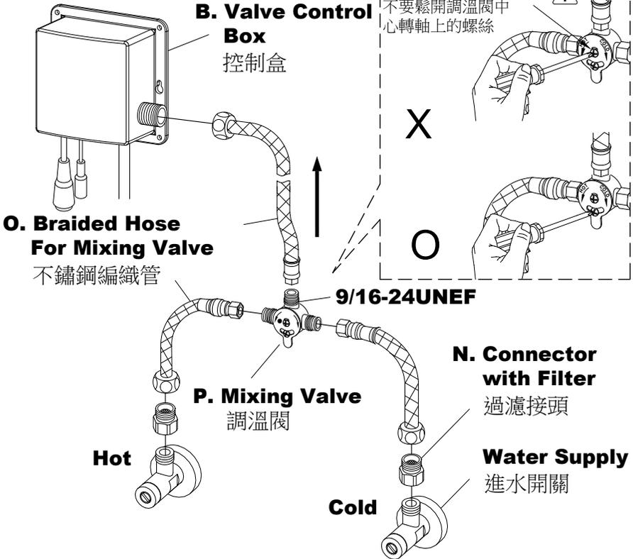
\* 1. After install faucet and **Valve Control Box**, connect **Valve Control Box, Mixing Valve** and Water Supplies with **Braided Hoses** and **Connector with Filter**.
