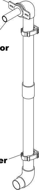
Keep the elbow of **PVC Pipe** be flush with finished wall.
