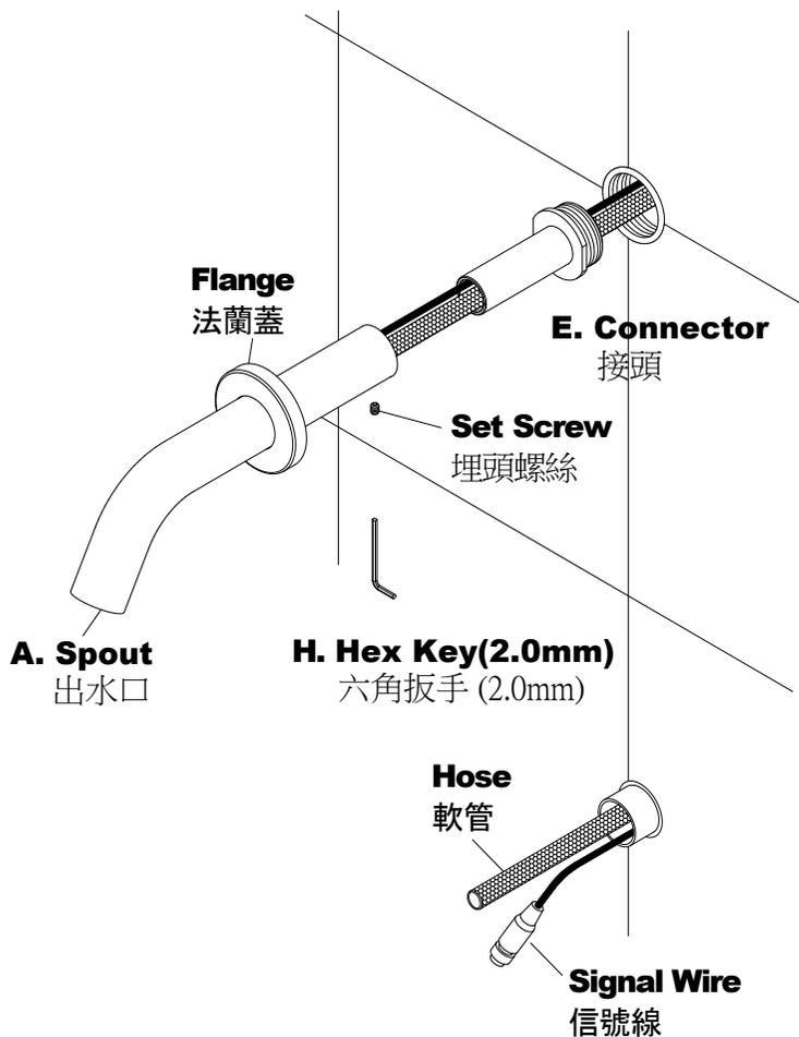
\* Screw **Connector** into elbow of **PVC Pipe**, and then insert Hose and Signal Wire into upper elbow of **PVC Pipe** and go out from the lower elbow. Slide **Spout** to the **Connector**, fix with **Set Screw** by **Hex Key(2.0mm)** securely, and then cover **Flange** on.
