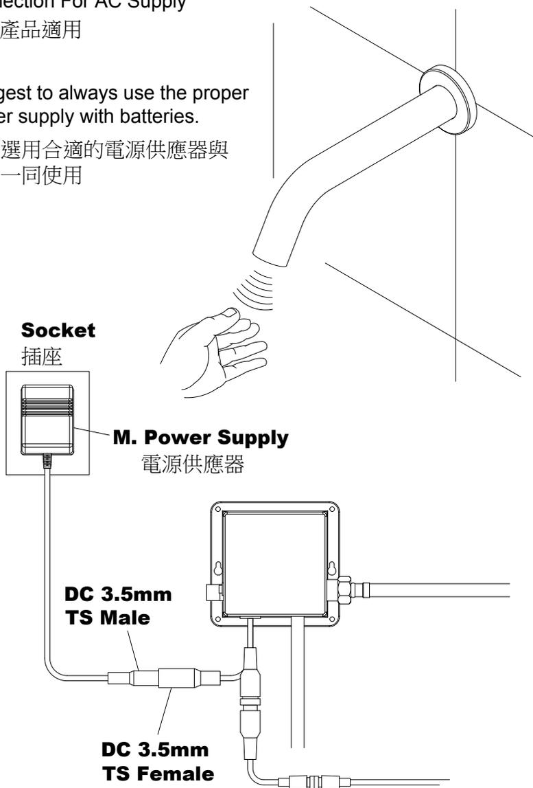
**\* Connect Power Supply to Valve Control Box and Signal Wire to faucet, and then test the Sensor.**
