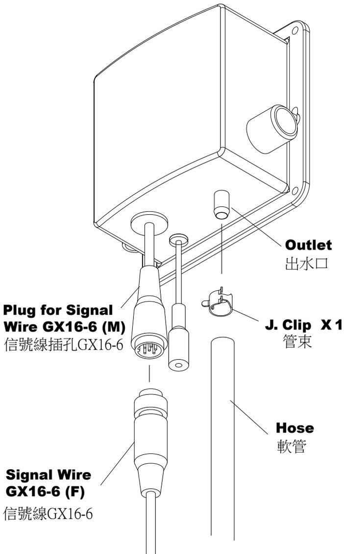
\* Connect Hose of **Spout** to Outlet of **Valve Control Box** with **Clip**, and connect the Signal Wire to Plug of **Faucet Body** and **Valve Control Box**.
