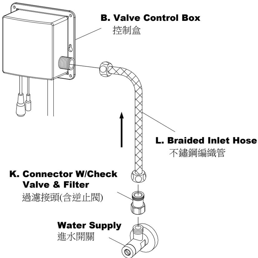
**\* After install faucet and Valve Control Box, securely connect Valve Control Box and Water Supply with Braided Inlet Hose and Connector W/Check Valve & Filter.**
