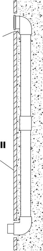
\* Use **Bracket** and **Pipe Holder** to help to fix and install the **PVC Pipe**, and please make sure to keep the elbow of **PVC Pipe** be flush with finished wall.
