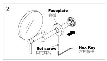
1. Loosen the Set Screw under the Faceplate with provided Hex Key, and move forward the Faceplate to gain the space of installation. Select the proper position for product and mark the centers of mounting holes on wall by using a spirit level and refer to the actual product for distance among holes.
