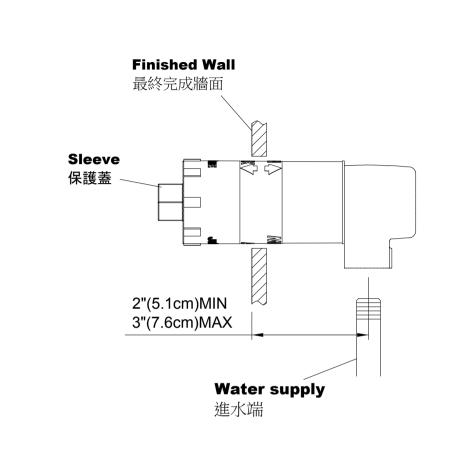
\* Connect hot and cold supplies pipes to the valve body, so they are between 2"(5.1cm) minmum and 3"(7.6cm) maximum from the finished wall; or keep the distance be 1.13" (2.9cm) to 2.13" (5.4cm) between top of cartridge and **Finished Wall** for necessary conditions.
