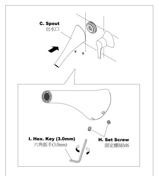
\* Position **Spout** onto **Base of Spout**, and then fix with provided **Set Screws** and **Hex Key**.
